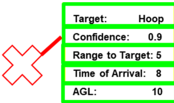
Figure 2: Symbology Example Metadata box and Red X for Target Identification, image referenced from Lockheed Martin DOMINANCE Kick-Off slides
